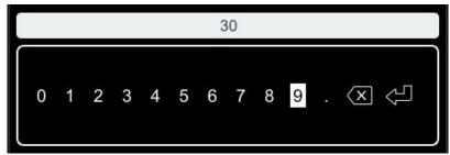
**Note:** If no settings are made on the numeric keyboard interface for more than 30 seconds, the instrument will automatically jump to the measurement display interface.
