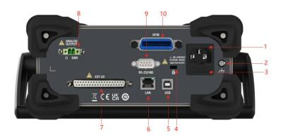
1 AC power socket 2 Shell grounding terminal
